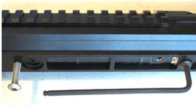
9: Now remove the longer screw from the rear hole and slip a 3/32" Allen wrench into this same hole and tighten down that short set screw that you installed in step #4. Try to tighten the set screw down without moving the Air Adaptor any. Tighten the setscrew down pretty tight, but don't strip it out!
