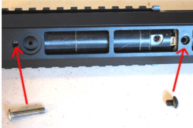
8: With both screws started, now tighten down the short front screw. There is a bit of "slop" in that hole. Even tho it is not critical, try to keep the screw somewhat centered in the hole as you tighten it.
