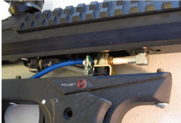
14: The trigger frame holds the Air Disk in place against the DTI4 body. Make sure the air disk does not get caught crooked as it is being assembled. It should flatten out on its own as the trigger frame is tightened down, but keep an eye on it as you attach the trigger frame.
