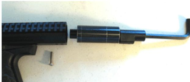
3: To re-install, simple reverse the removal steps. Take note that when starting the rear trigger frame screw back in, you might need to leave the large 5/16" Allen wrench in the tail of the Air Adaptor to rotate it until the rear trigger frame screw starts into the threads. Forcing the rear trigger frame screw to go in if the Air Adaptor is not aligned up properly can result in cross-threading the Air Adaptor.
