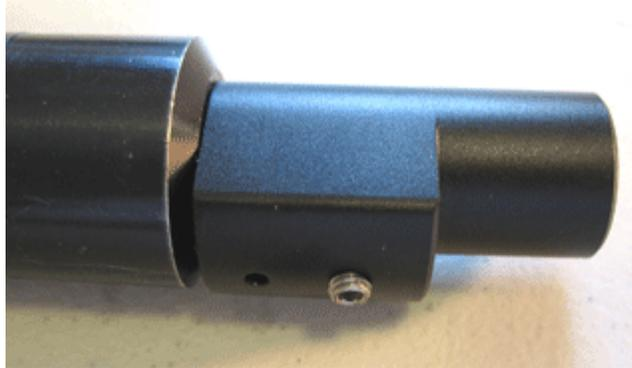
4: The Ion Breach and Fire Can thread together at a joint just behind the feedneck area. At this time, break this threaded joint loose (it might be tight!) and very lightly re-slug them back together. A very light snug, but not “sloppy”, connection is what we are looking for.
