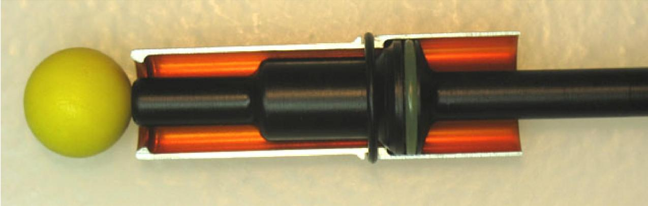
As the bolt moves forward, it cradles the ball with the deep cup face and minimizes "ball-stack-bobble". "ball-stack-bobble" is when there is a gap between the ball being chambered and the lip of the bolt. A gap here gives the next ball in the stack a place to blip down into between the ball and the bolt lip and can cause ball breaks and interfere with the bolt travel, causing inconsistent shots.
