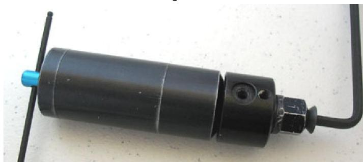
6) Slide the HP bolt tip onto the stalk as shown with the rubber insert facing forward. To ensure that the stalk is secured centered in the firecan, spin the firecan in your hand and watch the nose of the stalk. If the stalk moves around while it spins, then it might need to be "tweaked" some to get it centered. Simply push it the direction it needs to go. It might require a bit of force. Keep re-checking each time.
