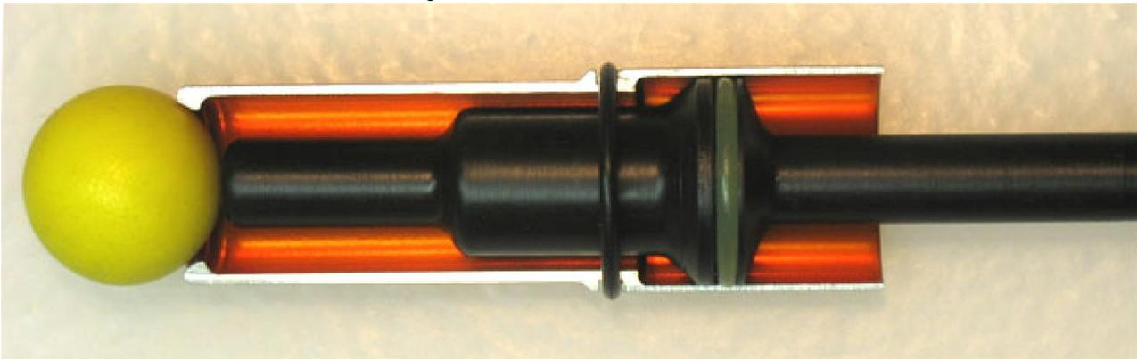
Near the end of the bolt stroke, the O-ring on the bolt stalk exits the bore inside the bolt and allows the air in the fire chamber to flow forward through the bolt. The HollowPoint is designed to try to maintain air flow consistency through the bolt for an efficient shot.
